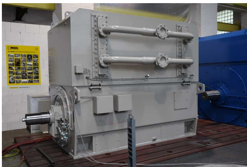
Caption: Menzel had a suitable replacement motor on stock and performed all electrical and mechanical adaptations as well as inspections inhouse
