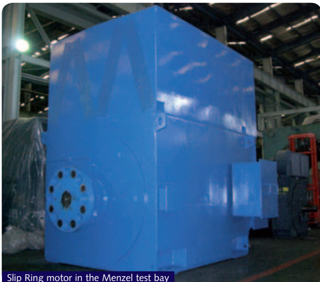
Slip Ring motor in the Menzel test bay
