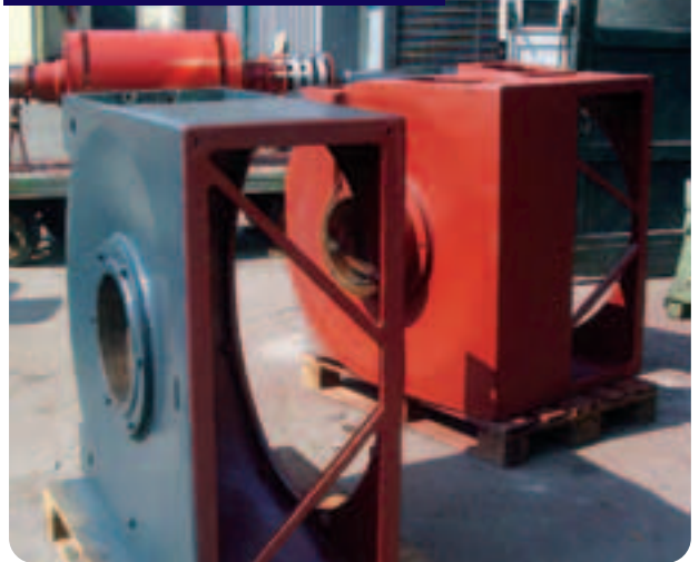
End shields with new holes in base and coat of anti-rust paint
