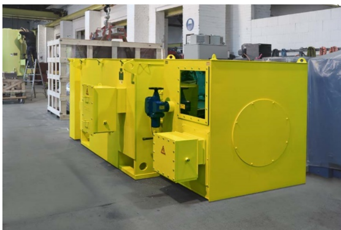
Caption: Menzel Elektromotoren has configured a slip ring motor with a short-circuiting and brush-lifting device for a cement mill
